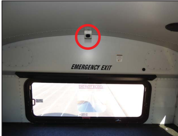
Figure 24: Surveillance camera in the back of the bus.
